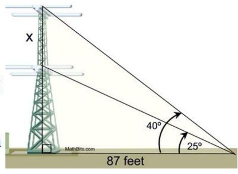
Smaller triangle with height a:  $\tan 25^\circ = \frac{a}{87}$ By  $a \approx 40.5687$ Difference (b - a)
